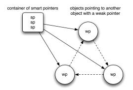
If the container of smart pointers is emptied, the three objects in the ring will get automatically deleted because no other smart pointers are pointing to them; like raw pointers, the weak pointers don't keep the pointed-to object "alive." The cycle problem is solved. But unlike raw pointers, the weak pointers "know" whether the pointed-to object is still there or not and can be interrogated about it, making them much more useful than a simple raw pointer would be. How is this done?
